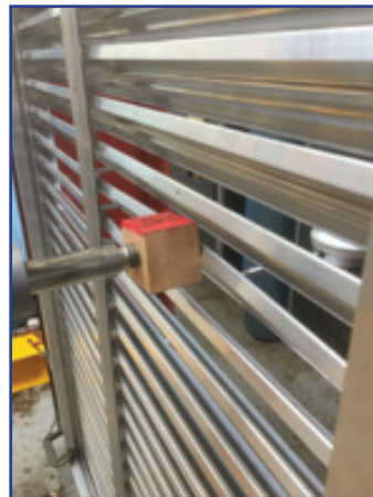
Point Load (Internal View of Test)
