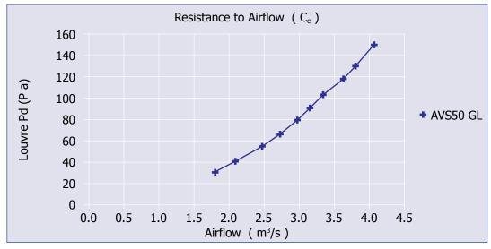
NB. The theoretical airflow rate is based on the face area of the louvre with the blades removed, and the coefficient is the measured airflow rate divided by the theoretical airflow rate
