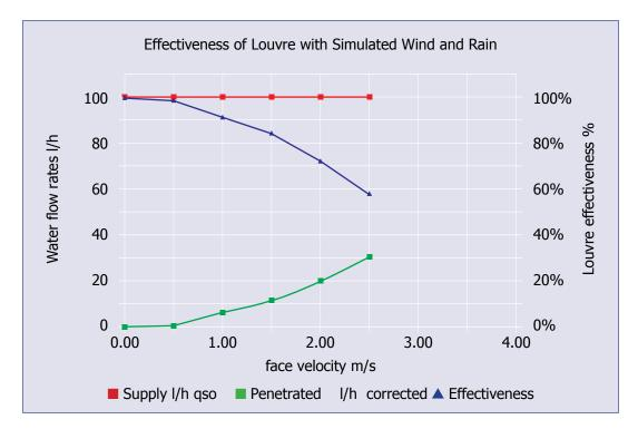
Performance testing is undertaken in line with BS EN 13030:2001 Ventilation for Buildings. Terminals. Performance testing of louvres subject to simulated rain.
